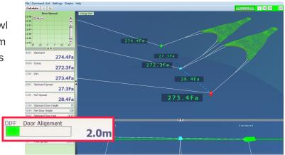
The Notus Trawlmaster Middle Wire Adjustment indicates the exact middle wire adjustment to align the clump with the doors, to ensure optimal fishing!
