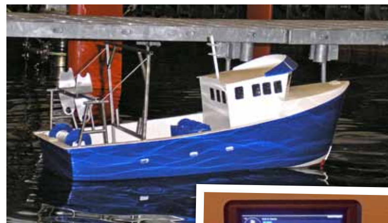
▲ Early tests of sensors and software were carried out using a wave tank and model.
